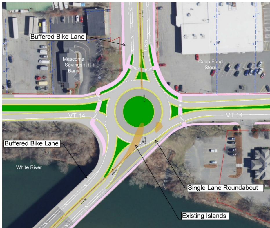
Figure 32 - Alternative LT5 - US 5/VT 14 Intersection Roundabout
